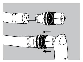
Secure friction fit adapter of the barrel to the tip of the endoscope, advance as far as possible. Note: Failure to do so may result in barrel dislodgement. Avoid bands while pushing. When placing the barrel onto the distal end of the endoscope, ensure trigger cord does not become pinched between the barrel and endoscope.
