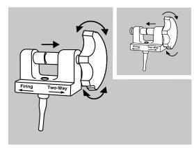
The firing position allows the handle to be rotated in the forward direction only. The two-way position allows the handle to rotate in both directions.
