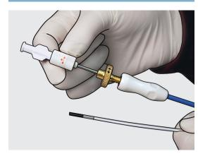
Disengage the Luer slip fitting from the adjustment wheel prior to adjusting the needle extension. **Caution:** Attempting to adjust the needle extension while the Luer slip fitting is engaged may result in damage to the device.
