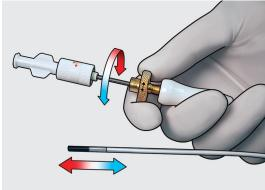
To adjust the needle, be sure to retract it back into the outer sheath before turning the adjustment wheel. Hold the device with the Luer lock fitting facing the operator and rotate the adjustment wheel clockwise to lengthen the needle extension, counterclockwise to shorten the needle extension.
